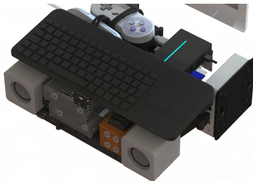
configuration B - 4 pi's and 1 Intel NUC
